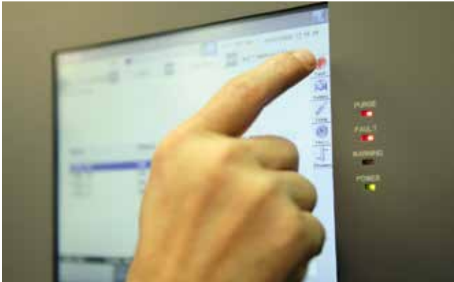
Fig. 5: Maxum Color Touch Screen Maintenance Panel
